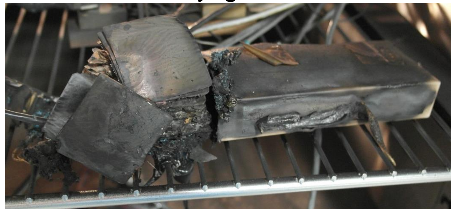
Photograph of a battery pack after a “thermal event”, where it is expected that a spark caused by a short circuit ignited the battery electrolyte.
